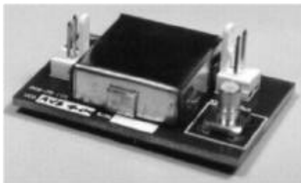
AVS400 VCO on Prototype board as supplied in Design Pack.
