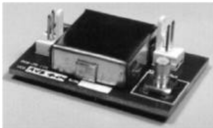
Typical VCO on prototype board as supplied in Design Pack.
