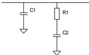
**Figure 1 - Passive Loop Filter**
