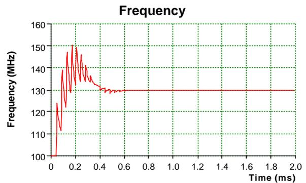
**Figure 2 - 100MHz to 130MHz Transient - no limiting**
